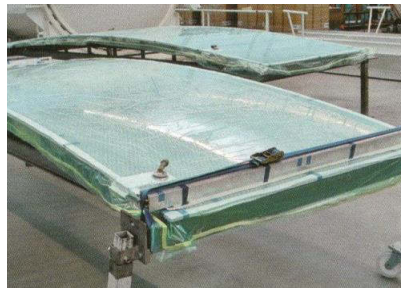
Figure 6 – Process of cold bending of glass (on the substructure, in the factory) [7]
