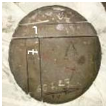
Figure 8. Photograph of the sample cut out from segment 4-1 of the upper ring of guide vane apparatus
