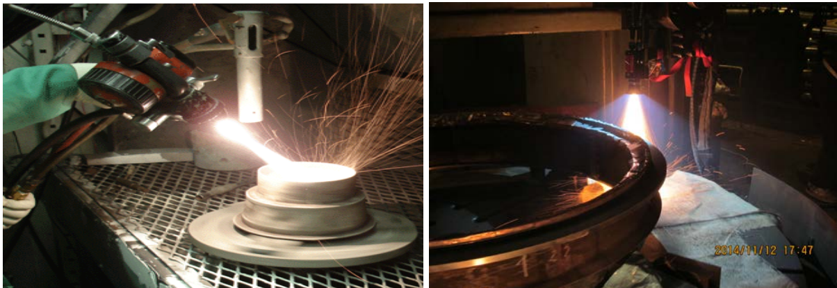
a) Appearance of the device for cold metallization b) Repair process of damaged surfaces of the flange
