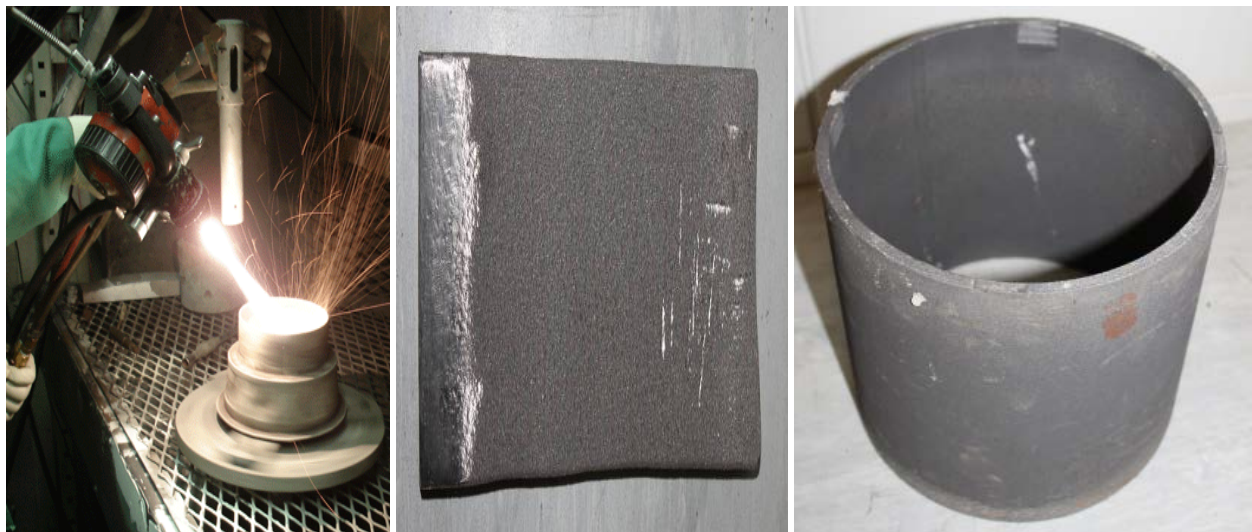
a) Device for metallization b) Appearance of the 12 mm thick metal sheet c) Appearance of the \text{\O}200 \times 6 mm pipe
