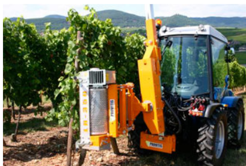
Fig. 9 Device for defoliation with perforated drum aggregated on the tractor from the rear side
