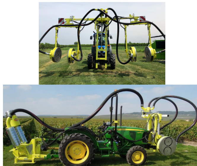
Fig. 2 a) device with a larger number of working heads; b) position of compressor and working head mounted on the front of tractor.
