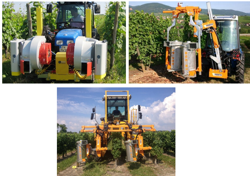
Fig. 1 a) defoliation device aggregated from the front of tractor; b) defoliation device aggregated from the rear of tractor; c) defoliation device aggregated on self-propelled machine
