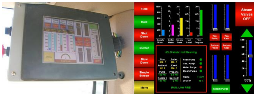
Figure 5. Control unit installed in the tractor cab
