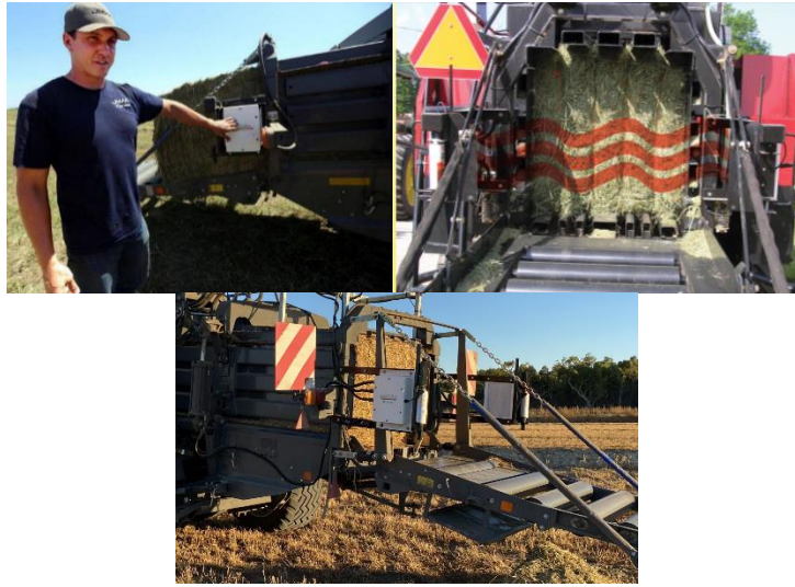
Figure 7. "Gazeeka" Device for measuring the humidity of the material installed on the press [34].
