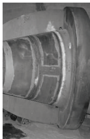
b) Improper mutual position of the collar and the anchor
