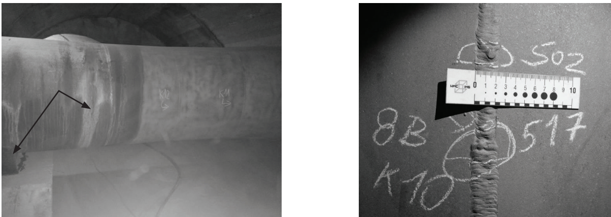
a) Characteristic damages that occur at parent material of the collar and the anchor
