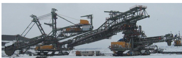
Figure 1. The bucket wheel excavator SchRs 1600 on the surface mine 'Tamnava West Field' (Serbia): theoretical capacity of 6600 m 3 /h, total mass (with the discharge bridge and loading unit) of 3344 t.
