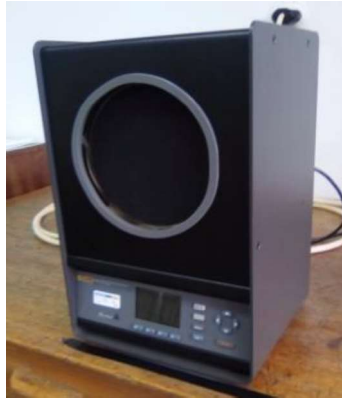
Figure 3: Source of thermal radiation
