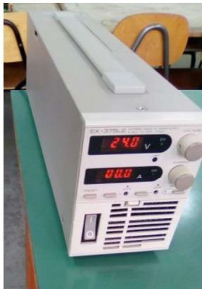
Figure 6: Infrared sensor power supply
