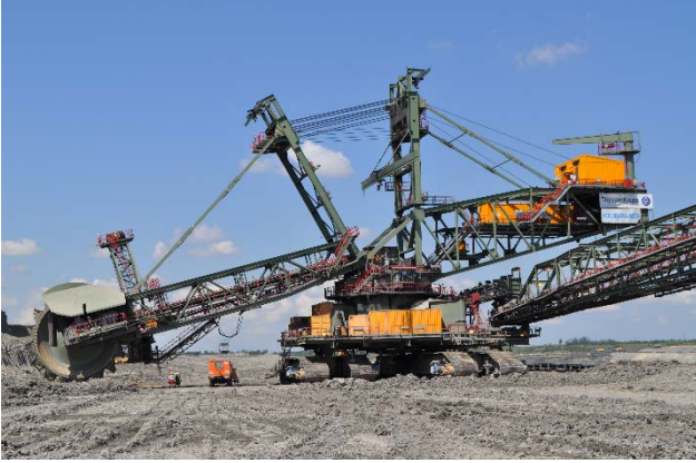
Fig. 1 BWE SchRs 1600 in the open pit mine “Tamnava West Field”- Serbia (total mass 2420 t)
