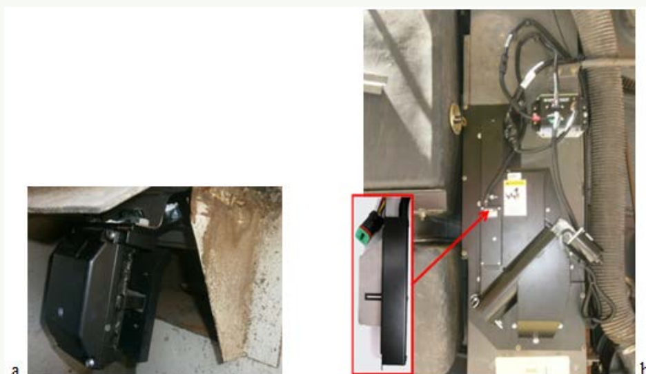
Fig. 2. a - Gape between elevator and auger for clear grain and impact plate of mass flow sensor with modul (view from grain tank) and b - grain moisture sensor
