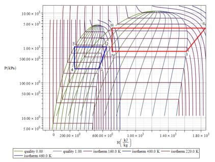
Figure 2 logp-h diagram of a cascade heat pump cycle
