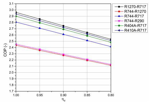
Figure 4 Analysis of the impact isentropic efficiency has on COP
