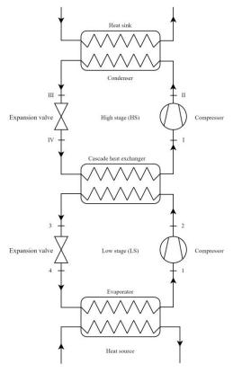
Figure 1 Cascade heat pump schema
