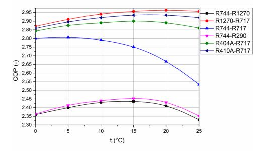
Figure 3 Results of the optimal intermediate temperature analysis
