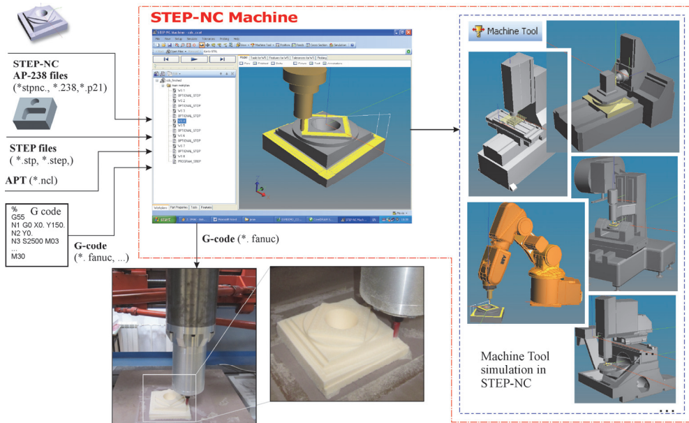
Fig. 4 Machining simulation in software STEP-NC Machine
