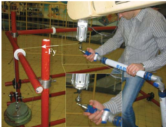
Fig.6. Experimental setup of robot loading and displacements measurement
