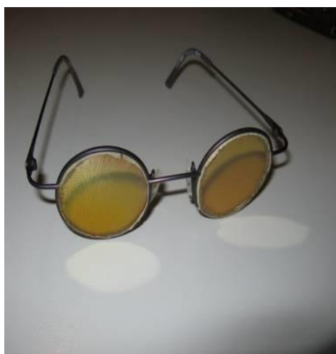
c) Filter 2. Debljina filma 60 nm
