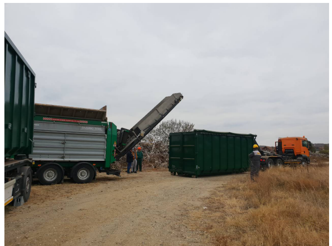
Figure 1: BEP's shredder machine processing waste wood from Danube river
