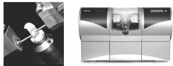
Fig.6. CEREC: 5-axis double tool milling system [12]
