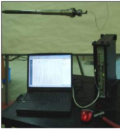
Fig.6. Measuring chain for the identification of dynamic system behavior spindle - tool holder - tool
