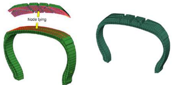
Fig.7. Typical mesh segment formed by assembling of body and tread segments. Nodes on contacting surface are tied by DOF coupling
