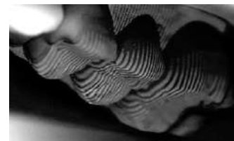
Fig.5. CEREC acquisition center: intraorally projected fringe pattern of short frequency visible light [12]
