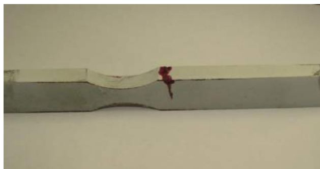
Fig. 8. Premature failure of test specimens due to casting defect - tested by liquid penetrants
