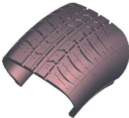
Fig.5. 3D parametric model of an existing tire type, dimensioned 165/70R13 [2]
