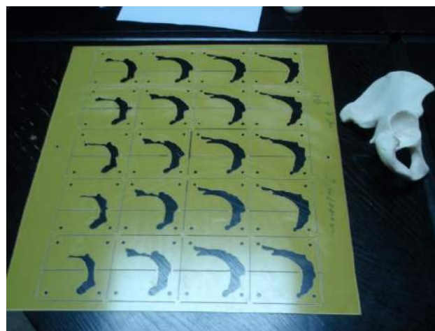
Fig.9. Different 2D cross-sections of Plexiglas material produced on the 3D milling machine
