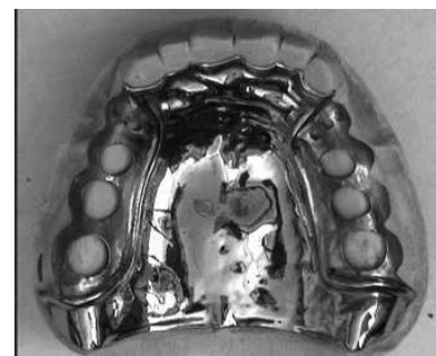
Fig.4 Partial upper denture-Ti6Al4V shaped by SPF [11]
