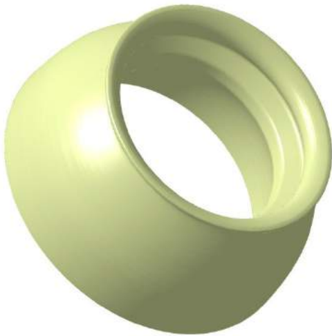
Fig.4. Reconstructed NURBS surface based on digitized data
