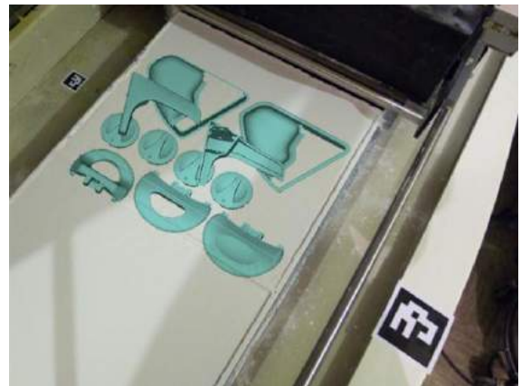
Fig.6. AR assisted part removal
