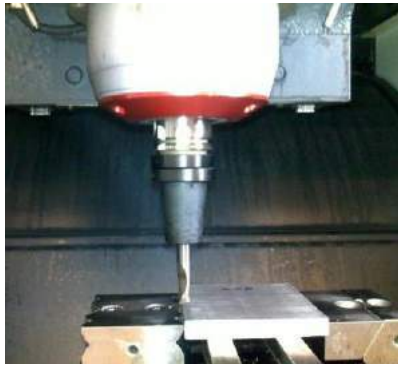
Fig.5. Cutting process on DMG Ultrasonic 20 linear machine tool with balanced tool arrangement by eccentric balancing rings on shrink fit tool holder with HSK 32 adaptor for high-speed milling.
