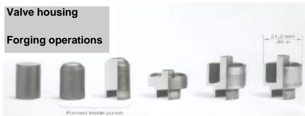
Fig 1. Forging workpiece and final part after four operations
