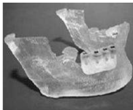
Fig. 2 Model of jawbone with a mounted drill guide, manufactured by stereolithography[7]
