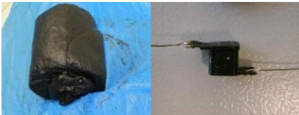
Fig.1. Raw conductive silicone rubber Elastosil R570/70 and one cubic sensor-specimen
