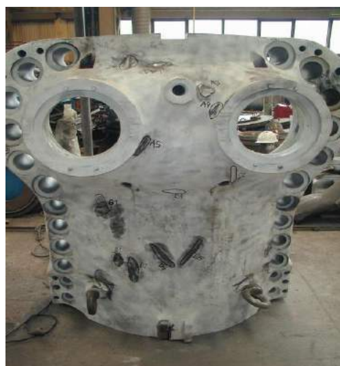
Fig 1. HP turbine casing, outer side
