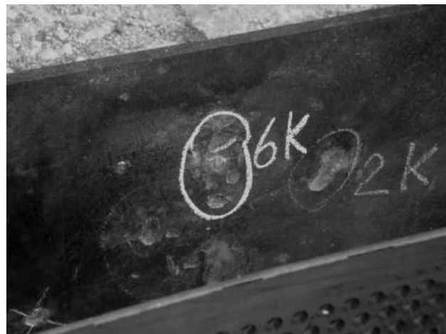
Fig.3. Five penetrating core fragments made smooth bulges on the basic plate [9].
