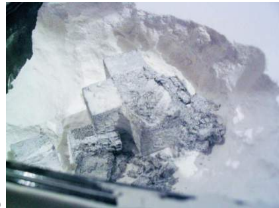
Fig.3. Part removal: a) vacuuming loose powder; b) damaged part due to improper extraction
