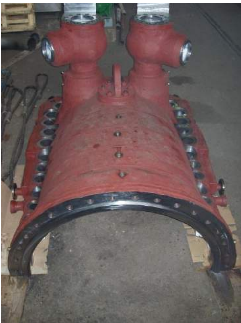
Fig. 4. HP turbine casing after revitalization
