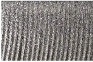
Fig.8. Cut surface generated in AWJ cutting of aluminium alloy sample
