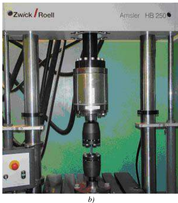
Figure 5. S-N diagram for 20GSL Casting a) S-N diagram b) Position of samples on testing machine
