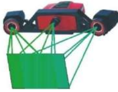
Fig. 2-6. Working principal of the ATOS II
