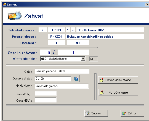
Fig.9. The appearance of form for defining operation
