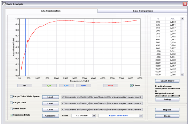
Fig. 11. Display of the sound absorption coefficient for a three-layer material, composed of 2 cm thick Ekomolitan positioned closer to the sound source and of 2 cm thick Nobasil and of 2 cm thick recycled rubber positioned at the end
