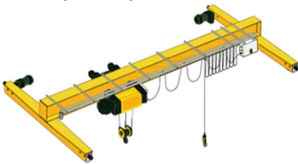
Fig. 1. Single Girder Bridge Crane
