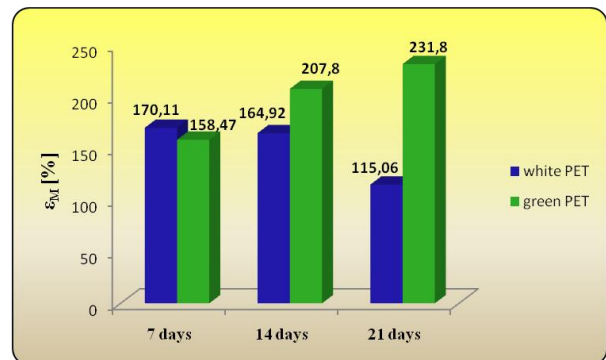
Fig. 11 The average values \epsilon_M of tested samples in environment of higher temperature
