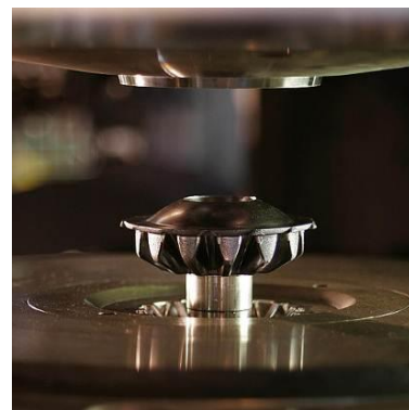
Fig. 3. Ejected gear after orbital forging
