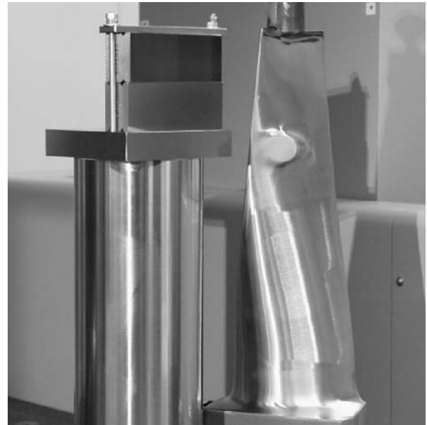
Fig. 3. MFG configuration (left) for the uncertainty assessment related to the turbine blade geometry (right) [2]
