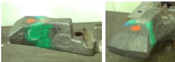
Fig. 3. Redesigned shape of cross members of scraper conveyor according to requirements of the customer
