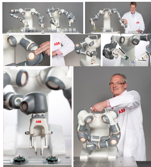
Fig. 1. Industrial dual-arm humanoid FRIDA ( Friendly Robot Industrial Dual Arm ) developed within EU FP7 project ROSETTA for safe cooperative work with humans on the lightweight products assembly lines. In addition to the requirement of small mass and high specific payload, industrial humanoid robot must have the inherently controllable compliance. This
