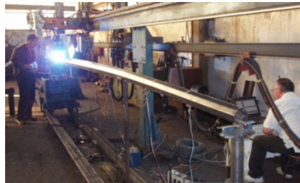
Fig. 3. Longitudinal conical pipe welding
