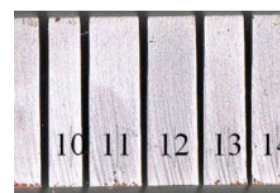
Fig. 6. The kerf geometry for different traverse speed
