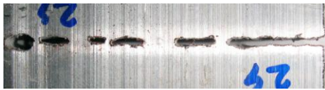
Fig. 5. Incomplete cut (view from the bottom side)
