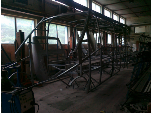
Fig. 3. Structure of bus
