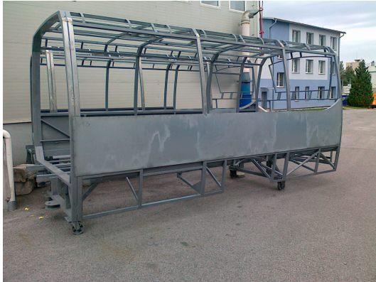
Fig. 4. Structure of bus
