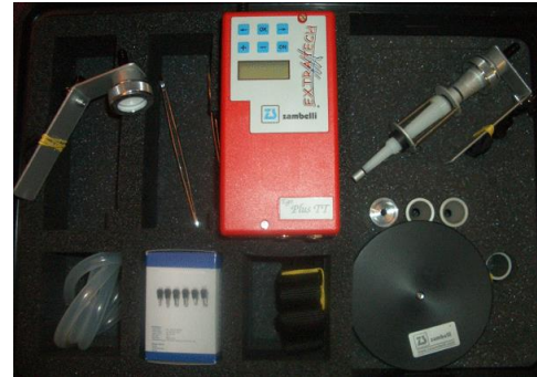
Fig. 1. Components of measuring instrument ZAMBELLI EGO PLUS TT.
