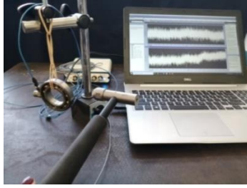
Fig. 2. Experimental modal analysis of ball bearings
