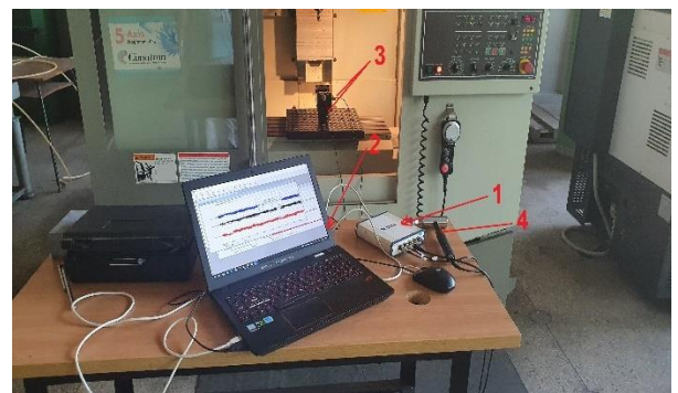
Fig. 4. Measuring system: 1- National Instrument device, 2- Laptop, 3- Accelerometers, 4- Impact hammer
