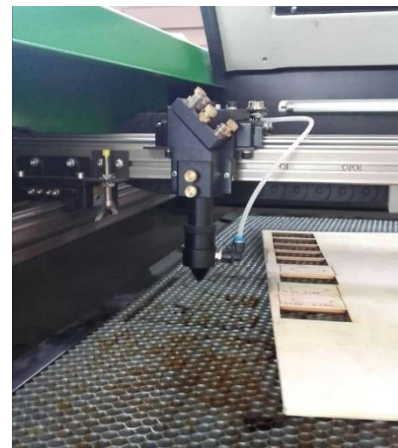
Fig. 3. CNC machine "LaserCut1209", working space and laser cutting head
