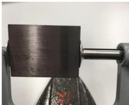
Fig. 1. Checking the bias of the measuring device by measuring the gauge block
