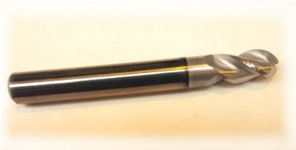
Fig. 2. Ball-nose end mill cutter used in machining
