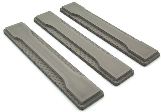
Fig. 5. Example of green parts printed via BMD in 17-4 PH stainless steel
