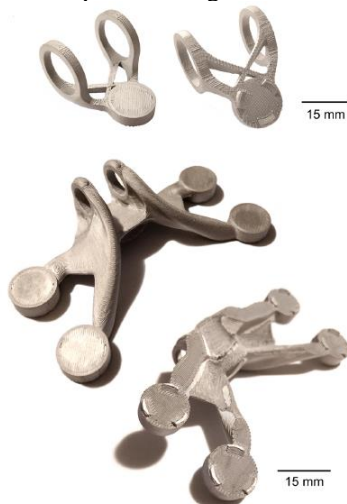
Fig. 2. Examples of parts made via ADAM in 17-4 PH [11]
