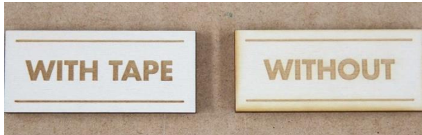
Fig. 2. Samples cut with protective tape and without protective tape [5]
