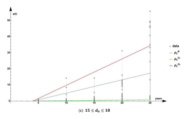
**Figure 3.** Linear models for the minimum (**a**), mean (**b**), and maximum (**c**) corrosion wear percentage of the LG ship structures.
