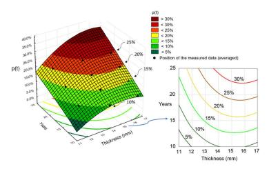
**Figure 5.** Corrosion depth percentage plotted against the operating time and built-in thicknesses of the LG of the bulk carriers examined.
