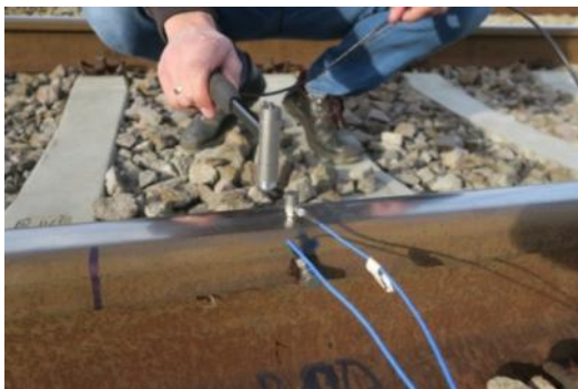
Fig. 4. Instrumented hammer impact for direct FRF
