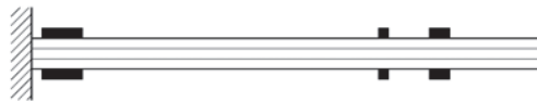
Figure 5. Beam with piezoelectric sensors and actuators which corresponds to the second case
