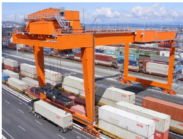
Figure 1: Rail mounted gantry crane at container terminal
