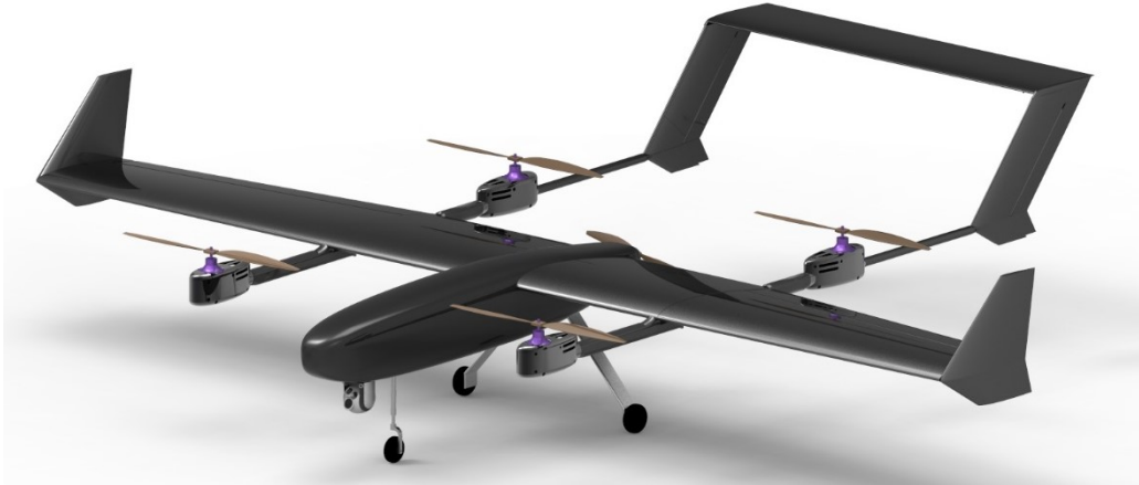
Fig. 4. The 3D model of the ALECS VTOL UAV.
