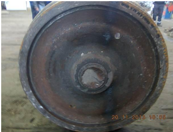
Fig. 2. Appearance of the railway axle fracture location
