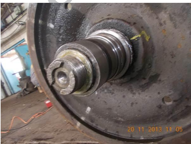
Fig. 3. Journal on the side of the railway axle where fracture has not occurred
