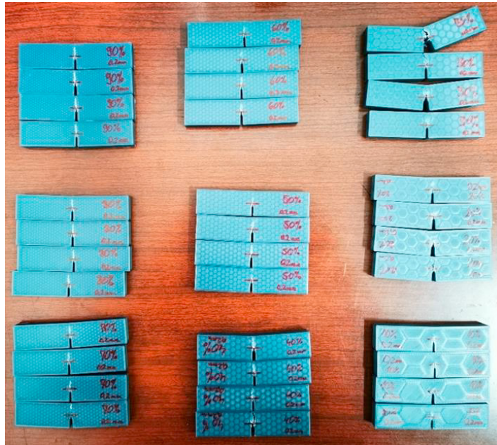
Fig. 2. Nine out of ten SENB specimen batches used in this research.
