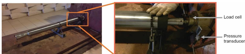
Figure 11. Static test equipment: pressure transducer and load cell
