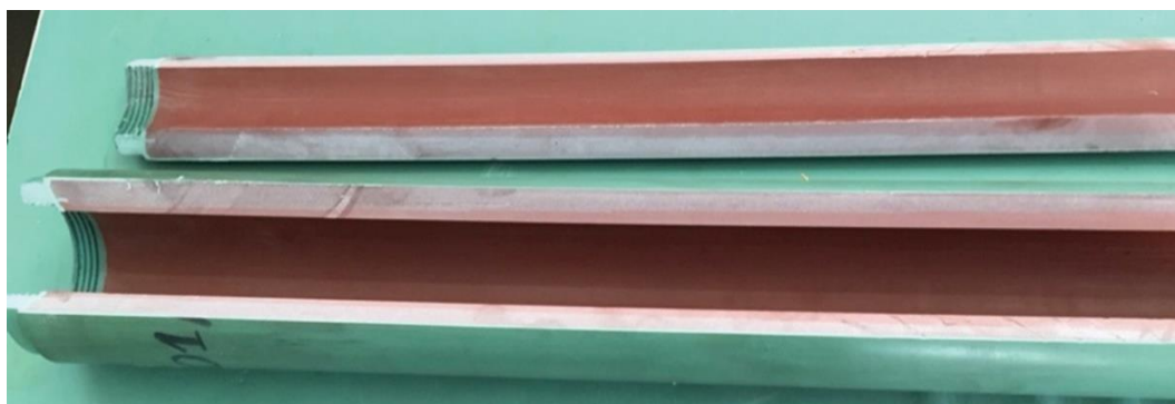
Figure 10. A cut out of the original model of the propellant grain
