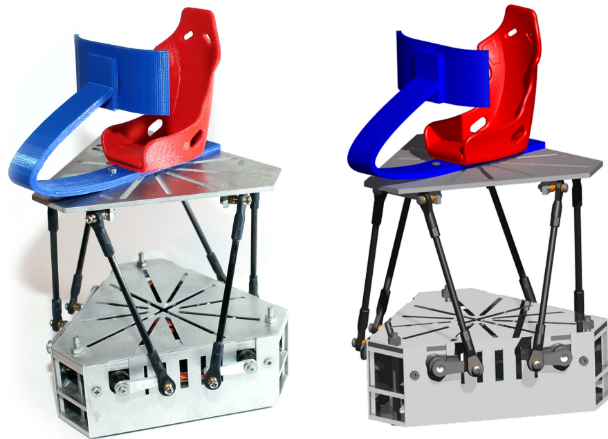
Figure 18. Scaled-down prototype of the mechanism (physical and 3D model).
