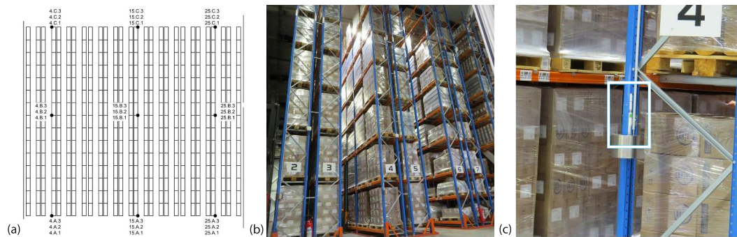
Figure 1. Data loggers positions (a), pallet racks (b), and detail view of data logger (c) (in rectangle)
