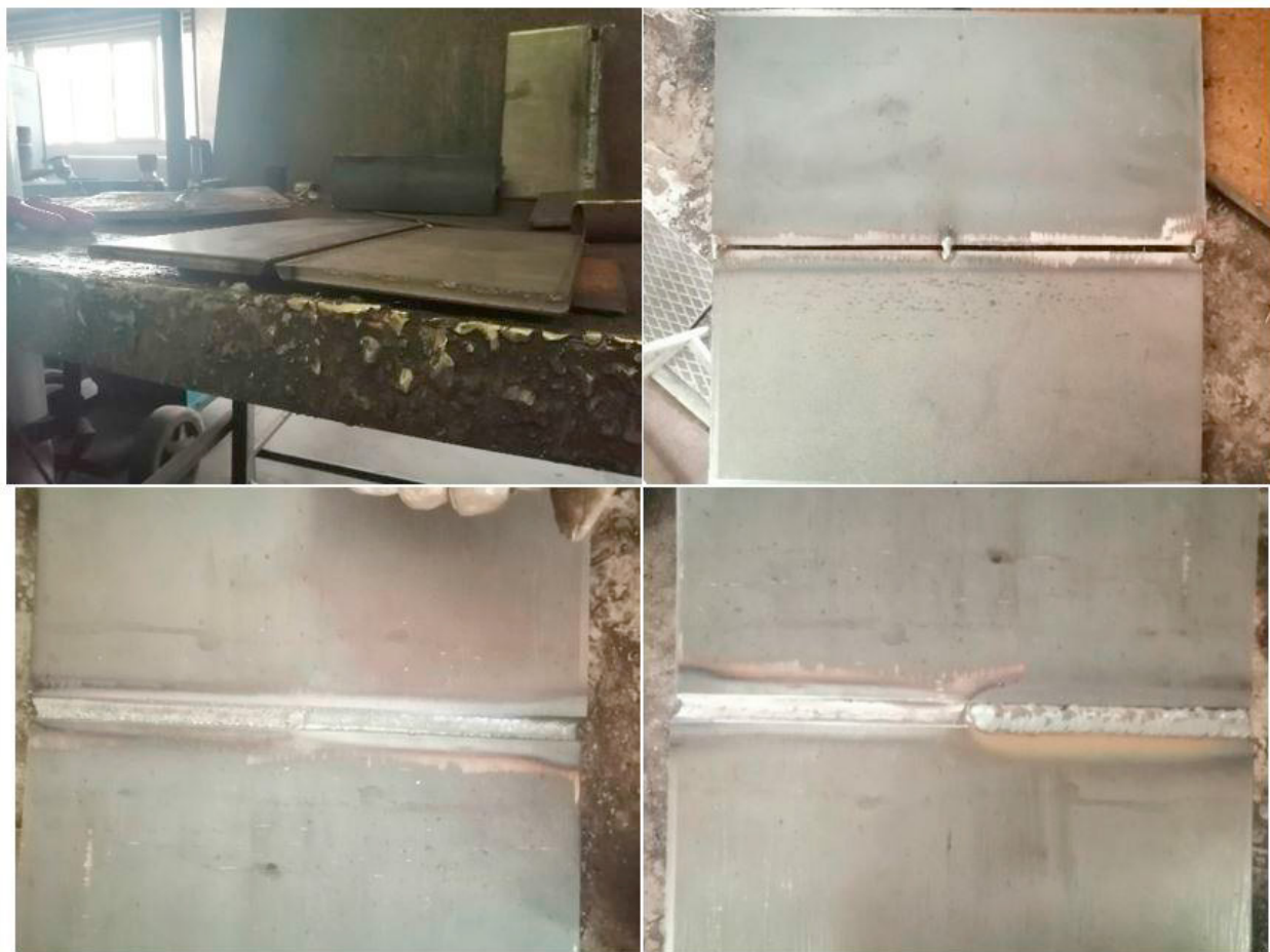
Figure 1: Welding of the plate with a misalignment
