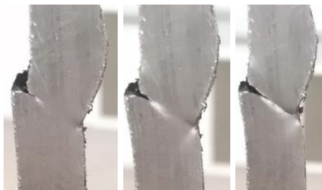
Figure 7. Welded joint specimen under tensile loads at different stages of the experiment.
