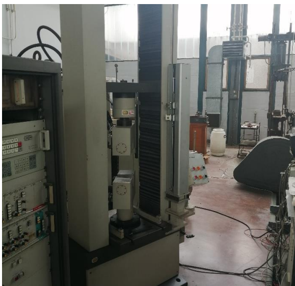
Figure 2. INSTRON tensile test machine of 250 kN capacity.
