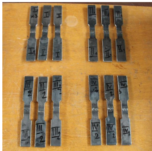
Figure 3. Tensile test specimens (all four groups).
