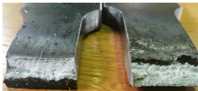
Figure 8. Model with excess weld metal, incomplete root penetration and an undercut.
