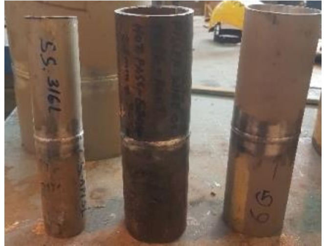
Figure 4. Butt weld joint CS-SS, CS-CS and SS-SS.
