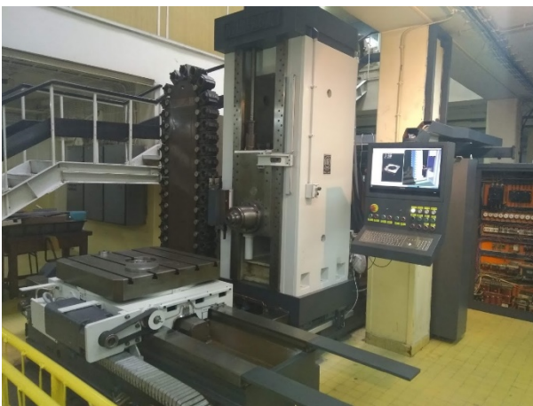
b) Retrofitted machine LOLA HBG 80 V3 with Linux CNC control system
