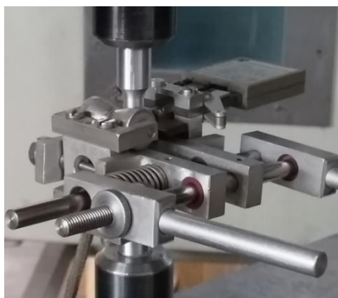
Figure 1. Specimen with extensometer, prepared for testing.
