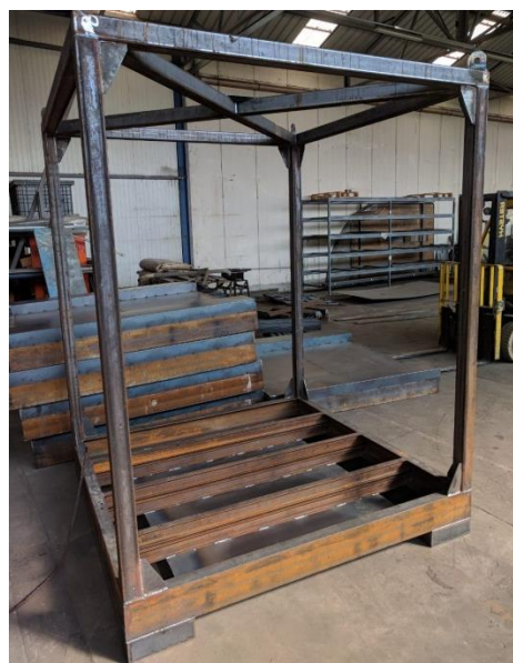
Figure 10. Initial stage of the base assembly.
