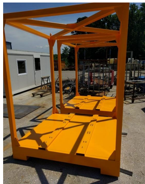
Figure 11. Final stage of the base structure assembly, including the floor plates.
