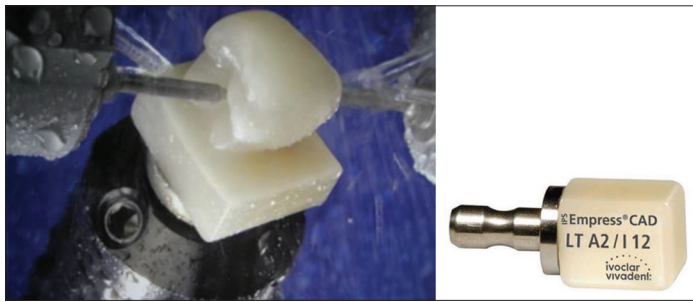
Figure 7. Left – the action of milling a ceramic crown in an in-office CAD/CAM machine; right – a ceramic block from which the ceramic crown is milled
