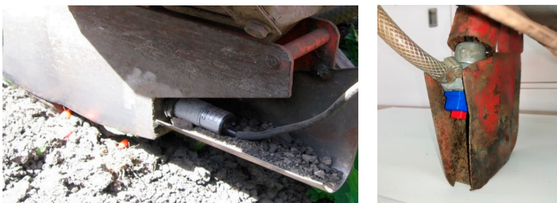
Figure 4. Photo electric sensor and the electric injector (Source: Original).
