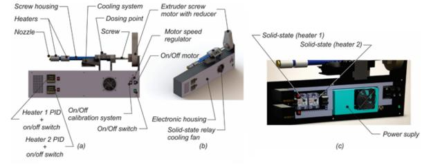
Fig 2. Design of filament extrusion system for recycling process in (a) frontal and (b) isometric view, with (c) internal cross section
