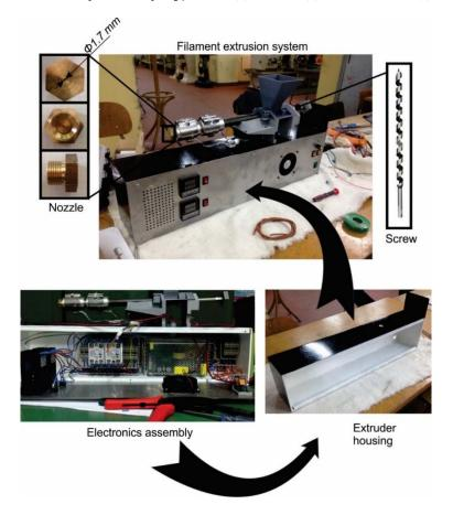
Fig 3. Assembly of filament extrusion system for recycling process
