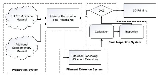
Fig 1. Schematic of the concept of FFF/FDM material recycling
