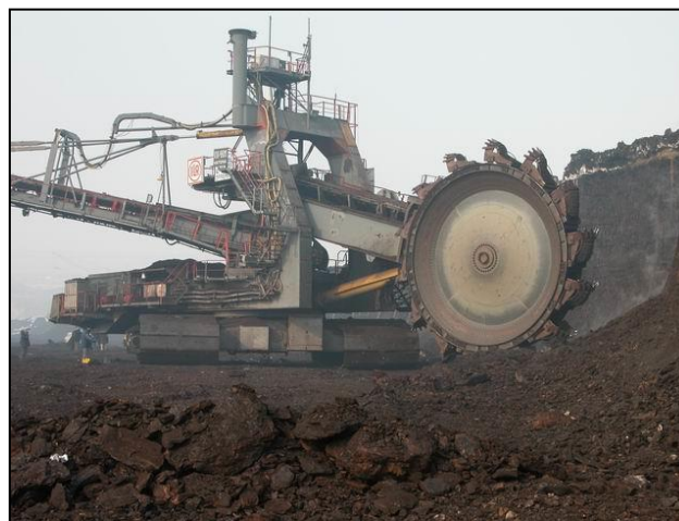
Figure 4 Rotary excavator SchRs 800.15/5 in operation
