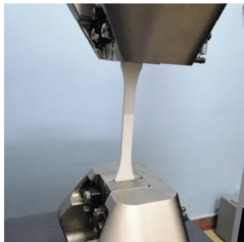
Fig. 4. ISO 527-2 specimen on universal tensile testing machine.
