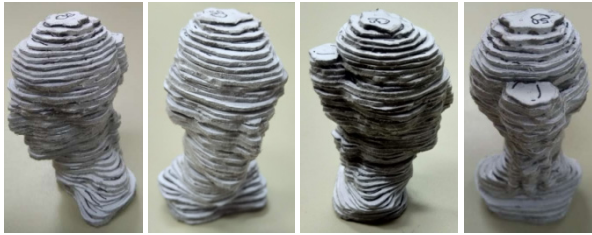
Figure 16. Model obtained by gluing layers of cardboard
