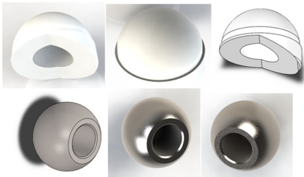
Figure 8. Final models of the metal spherical element and the polyethylene cup (different views and rendering)
