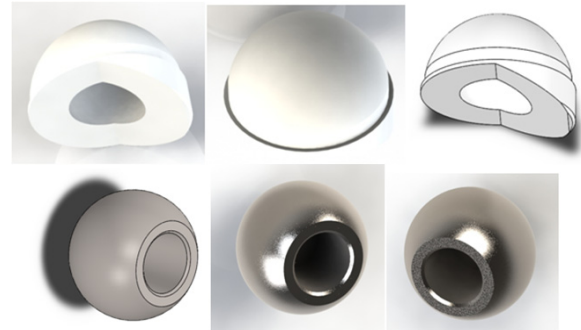
Figure 10. Final models of the metal spherical element and the polyethylene cup (different views and rendering)
