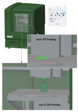
Fig. 8 Machine simulation in PTC Creo environment for toolpath of 3D printing
