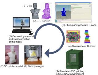
Fig. 4 Stages for additive manufacturing process from CAD model to 3D part
