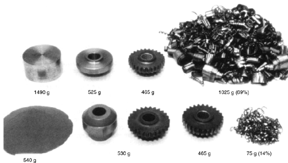
Figure 1. Comparison of materials used for conventionally forged cylindrical involute gear (top) and the equivalent powder forged involute gear (bottom).
