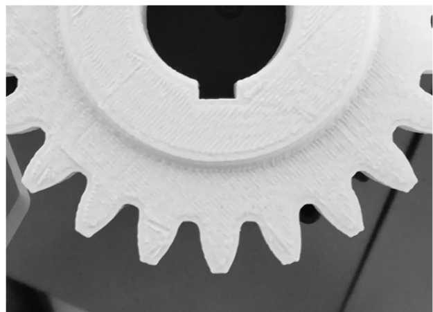
Figure 4. Successful printing of involute gear with 95% infill.
