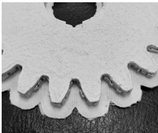
Figure 3. Unsuccessful printing of involute gear with 100% infill.
