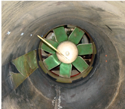
FIGURE 3. Measurements with a classical probe in a diffuser
