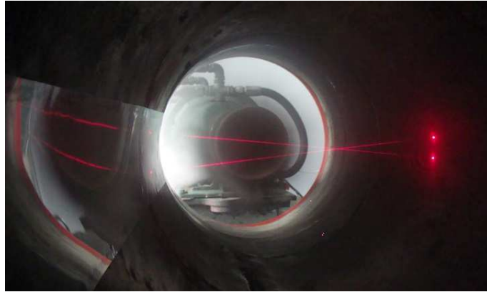
FIGURE 2. Laser Doppler anemometer measurements in a diffuser
