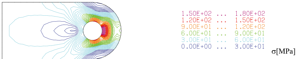
Figure 4. Representation of von Mises stress field ( \sigma ) with associated scale for connecting lug U1
