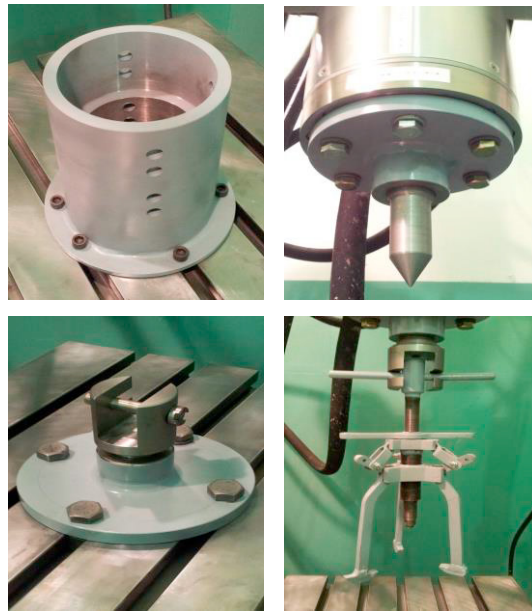
Fig. 7. Custom-made tools for the actual ejecting force testing
