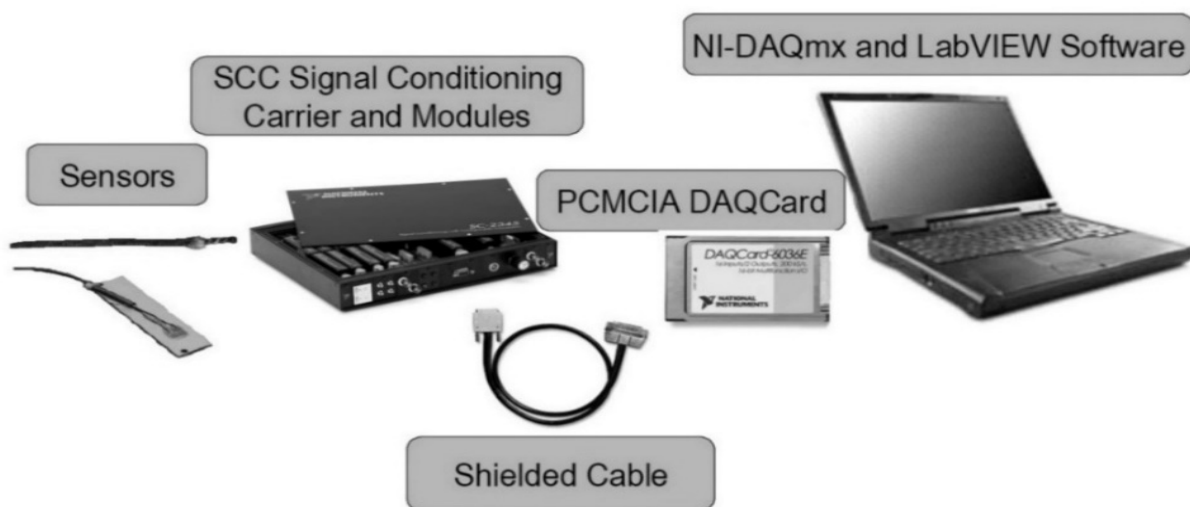
Fig.5. Acquisition rig – DAQ system used for monitoring friction torque and temperature
