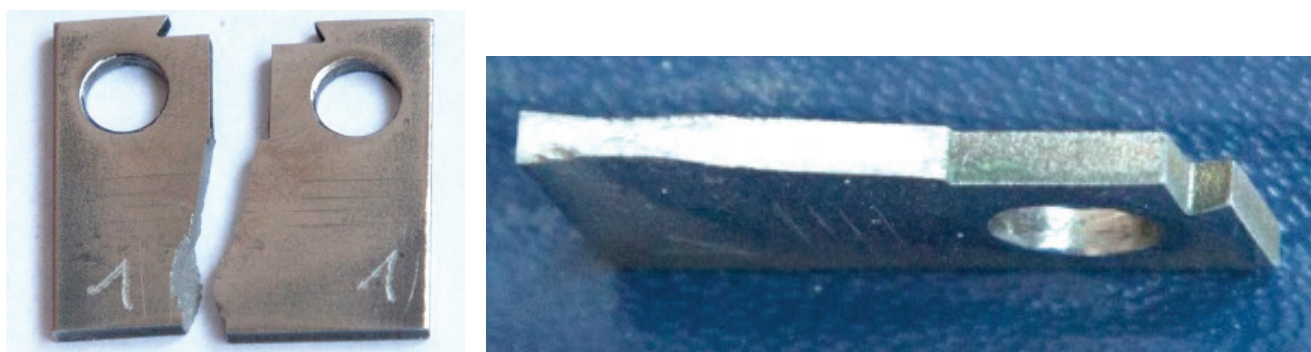
Figure 9. S316L specimen after fracture (left); fractured surface (right).
