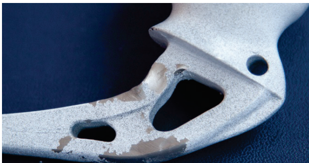
Figure 7 Plastic strains after static testing of hip implant
