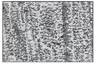
Figure 2 Micrograph of WM Magnification 200 x
