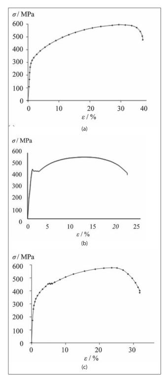
**Figure 5** Stress-strain curves for base metals and welded joint as the whole
